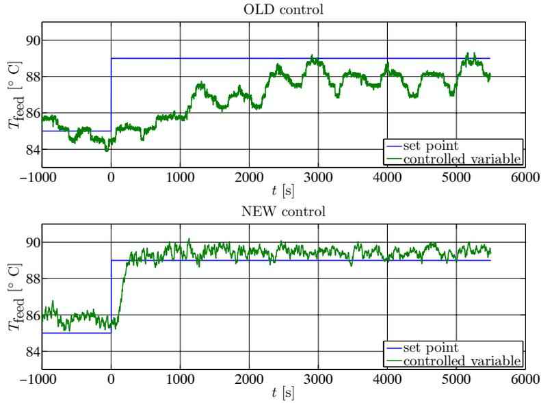
Figure 2: Feed temperature at a stepwise increase of the set point for the feed temperature
