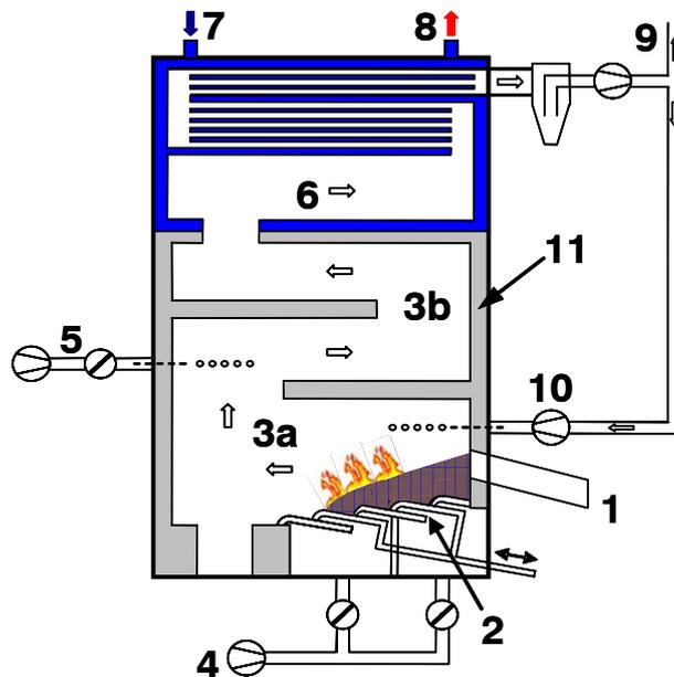
Figure 1: Pilot-scale furnace of the BIOENERGY 2020+: 1 ... fuel feed, 2 ... grate, 3a ... primary combustion chamber, 3b ... secondary combustion chamber, 4 ... primary air, 5 ... secondary air, 6 ... heat exchanger (boiler), 7 ... return, 8 ... feed 9 ... flue gas, 10 ... flue gas recirculation, 11 ... refractory lining
