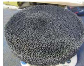
**Figure 2:** Porous burner (8-10 PPI) as used for the test run for the model validation
