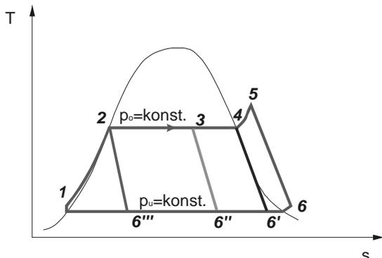
**Figure 3:** Possible cycles of operation of the screw-type engine process
