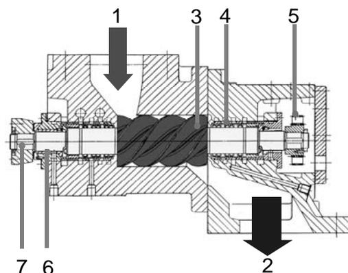
**Figure 1:** Section drawing of a screw-type engine
