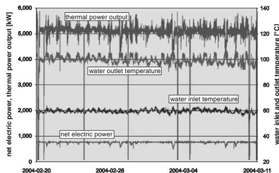
**Figure 9:** Relevant operating data of the biomass CHP module in Hartberg measured during the monitoring period
