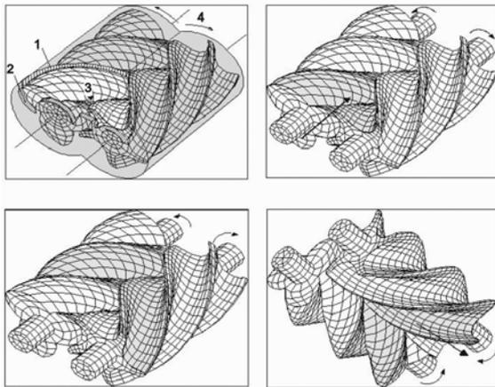
**Figure 2:** Expansion process within a screw-type engine
