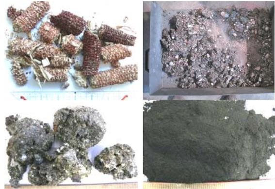
**Figure 2:** Pictures of the fuel applied and different ash fractions
