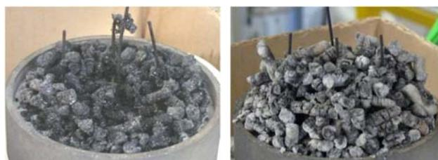
**Figure 5:** Pictures of the residues (ashes) after the test runs with wheat straw (left) and with a wheat straw/kaolin mixture containing 4 wt% kaolin (right)
